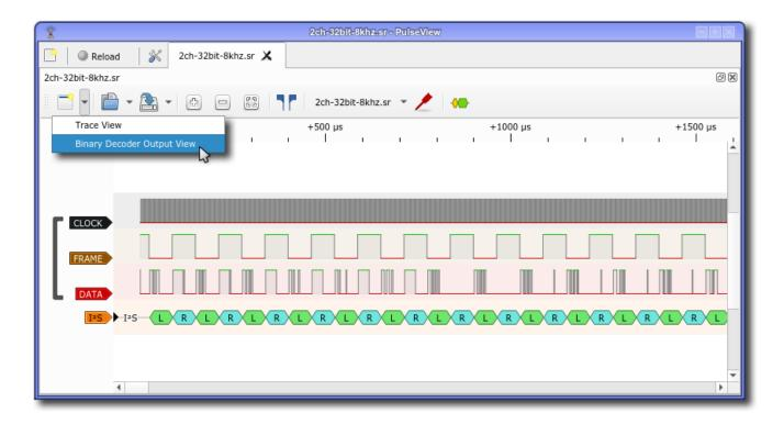
Once opened, you need to select a decoder with binary output for it to show anything - among which are I2C, I2S, EEPROM24xx, SPI and UART. Having acquired some I2S data and using the I2S protocol decoder lets you have the sound data as raw .wav file data, for example:
