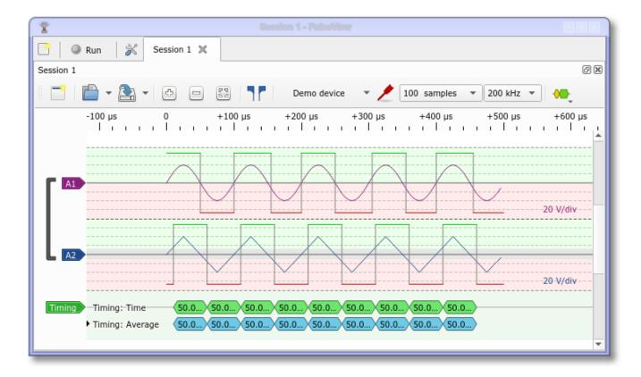
Here, A1 has been converted using a threshold (with default settings) and A2 has been converted using a Schmitt-Trigger emulation (also with default settings). Additionally, the conversion threshold display mode has been set to *Background* in the *Views* settings dialog. This way, you can tell how PulseView decided to change the logic signal level as you can now visually understand where the ranges for high and low are placed.
